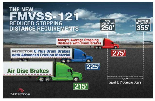
Product enhancements have reduced the gap between air drum and air disc brake performance
